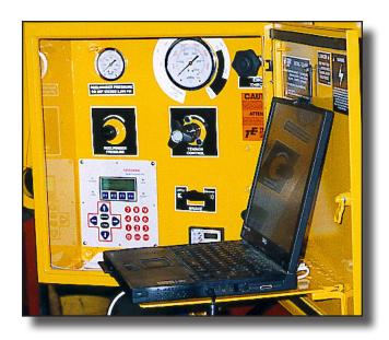
Digital display of: linepull, speed, distance and operator adjustable preset maximum linepull.
